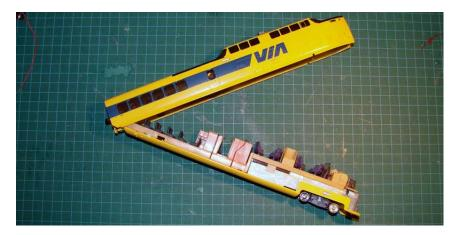
Align and slide the back part of the interior and floor into the back part of the shell to get the process started. Then, slide the front part of the interior and floor in. You may need to help the tabs seat into their sockets by pressing on the sides of the shell.
