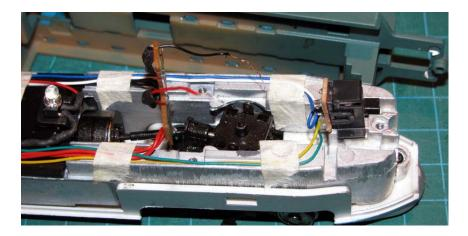
Once you have the wires undone, you can then proceed to removing the gearbox. Start by removing the screw holding the weight in place – it is right at the front of the unit.
