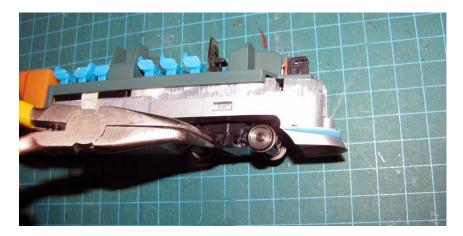
The final step is to reinstall the nose. Start by placing the bottom tabs on their seats in the shell, and then snapping the top into place.
