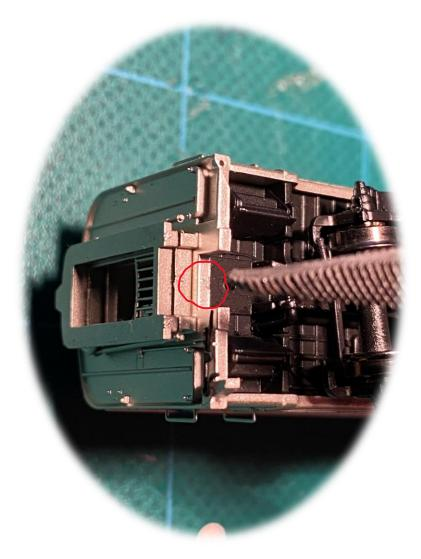
3. Install the coupler screw back in, making sure that your screwdriver is straight up and down – or even towards the front at a slight angle to compensate for the improper installation. (If you tighten it too much, the coupler may not swivel freely but can be fixed by loosening the screw ever so slightly until movement is free side to side).
