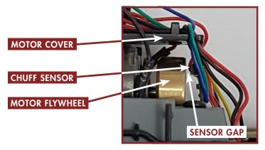
**6.** Cut a thin card (a business card is perfect) into a rectangle about 5mm x 40mm in size. Wedge this card between the flywheel and the sensor on the board (see "sensor gap" at left).
