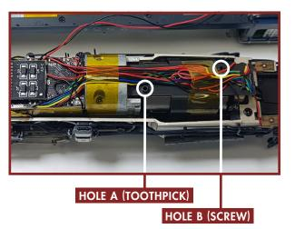
**9.** Once set, remove the card wedge, place the shell on the boiler (you may screw it back in once you have tested the result) and test the Hudson.
