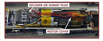
**5.** The intermittent chuff or total loss of chuff is because the motor top cover has shifted from it's locked position due to a play in the locking tabs. This moves the sensor board too far away from the magnetic contact on the flywheel, resulting in partial or complete loss of chuff sound.
