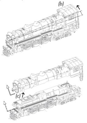
boiler top can be slowly lifted straight up and clear of the chassis. Why slowly? Because of even more wires! The *Empress* ditchlights are especially delicate.
