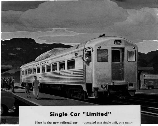
Here is the new railroad car which is a train in itself—the self-propelled, diesel-powered, all-stainless steel RDC-1. The Budd Company created it to perform a service both to railroads and their patrons, by carrying more passengers on short or long hauls at lower operating cost.
