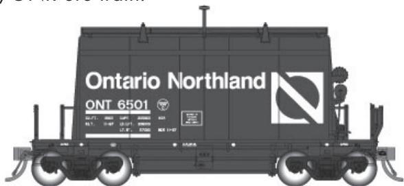
This train plied the rails from two mines owned by Dofasco in Northern Ontario to their facility in Hamilton, Ontario. At first glance the cars look like a shrunken cylindrical hopper. The reason for the round shape and covered hatches was to keep the
