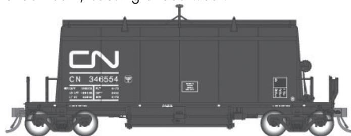
Also unique is the "tire" that sits on top of the hatches. At the loadout, the tire comes into contact with a "scroll" that forces the hatches to open - taking 60 seconds to fill a car and roughly an hour and twenty minutes for a unit train of 40 cars. Many times one could see CN and ONR cars mixed in a consist.
