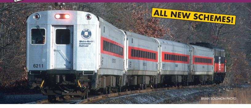
Introduced by Pullman-Standard as a replacement for aging commuter cars, the soon nicknamed "Comet" cars were first built between 1970 and 1973 for the Erie-Lackawanna Railroad's services out of New Jersey.
