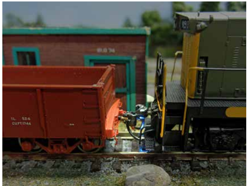
Note the blue light reflecting off the coupler. LED is only illuminated when uncoupler is in the 'ON' position.
